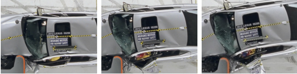
Figure 8 Example of Excessive Head Lateral Movement — 2012 Lexus IS 250 (CEN1205)
