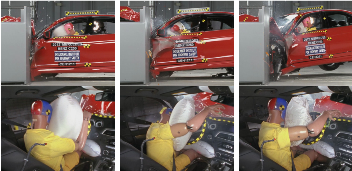
Figure 3 Example of Partial Frontal Airbag Interaction — 2012 Mercedes Benz C250 (CEN1211)
