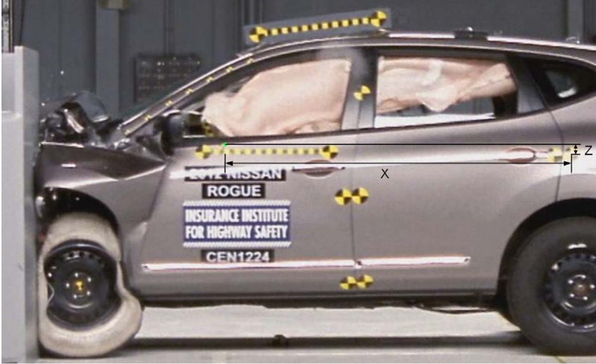
Figure B-3 Marking Steering Wheel Center on Door, Mid-Crash
